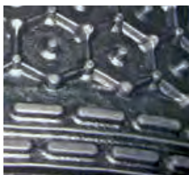
sealing lips on lower side
