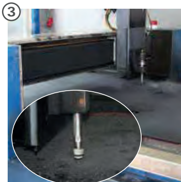
based on the CAD created drawing, the slits are cut exactly into the mats with innovative water jet technology
