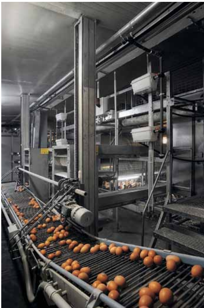
> Egg Lift collection system - "Anaconda" chain
