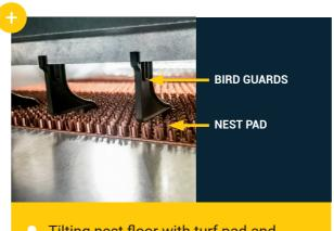
Tilting nest floor with turf pad and bird guards
