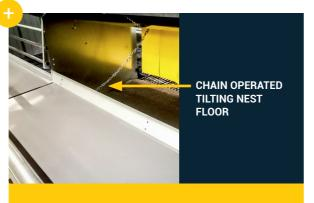
Low torque chain nest floor lifting
