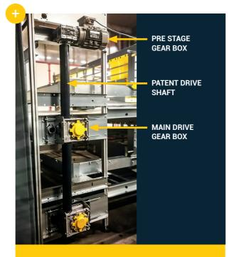
Separated pre and main drive gear box with patent shaft drive.
