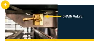
Oil drain valve at the main gear assembly for easy oil changes.
